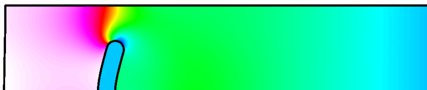
Figure 8.3: Pressure distribution of the obstacle in channel case.
